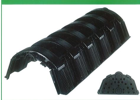
The High Capacity Infiltrator Chamber offers maximum volume per linear foot for extra temporary storage capacity. The 10" louvered sidewalls facilitate infiltration and evapotransporation. With 12" of compacted cover, it supports 16,000 lbs/axle, equivalent to an H-10 AASHTO rating.
